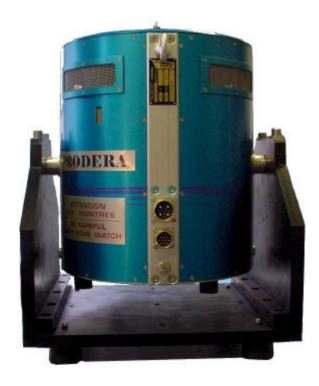
The trunnion type BF 520 has been developed to allow a stable support for the shaker type EX 520 C50. It can be directly installed on its rubber feet to operate at relatively high frequency and it must be securely attached for low frequency tests. The trunnion BF 520 is also designed to be suspended by one or four attachment points by means of elastic cords or springs.
