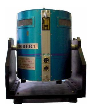
The trunnion type BF 320 has been developed to allow a stable support for the shaker type EX 320 C50. It can be directly installed on its rubber feet to operate at relatively high frequency and it must be securely attached for low frequency tests. The trunnion BF 320 is also designed to be suspended by one or four attachment points by means of elastic cords or springs.
