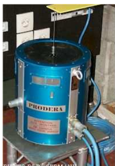
EX 520 C50 Long stroke shaker (550 N)
