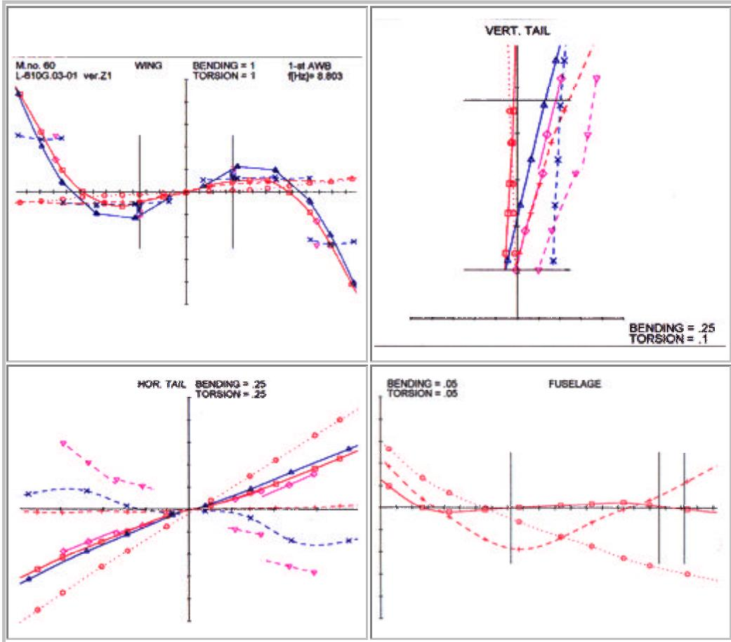
Figure 6 - Deform lines of antisymmetric first wing bending of L-610G aircraft
